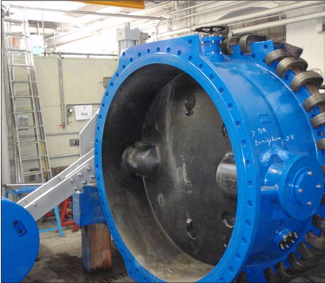
VAG EKN® 78" Butterfly Valve with HYsec Hydraulic Brake-and-Lift Cylinder during customer acceptance the pressure test in 2009 at a power plant in Boxberg, Germany.
