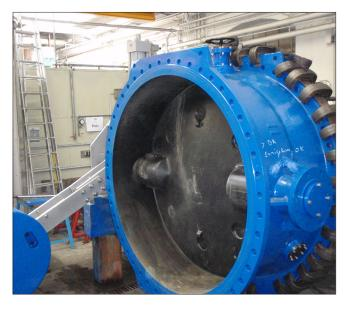
VAG EKN® 78" Butterfly Valve with HYsec Hydraulic Brake-and-Lift Cylinder during customer acceptance the pressure test in 2009 at a power plant in Boxberg, Germany.
