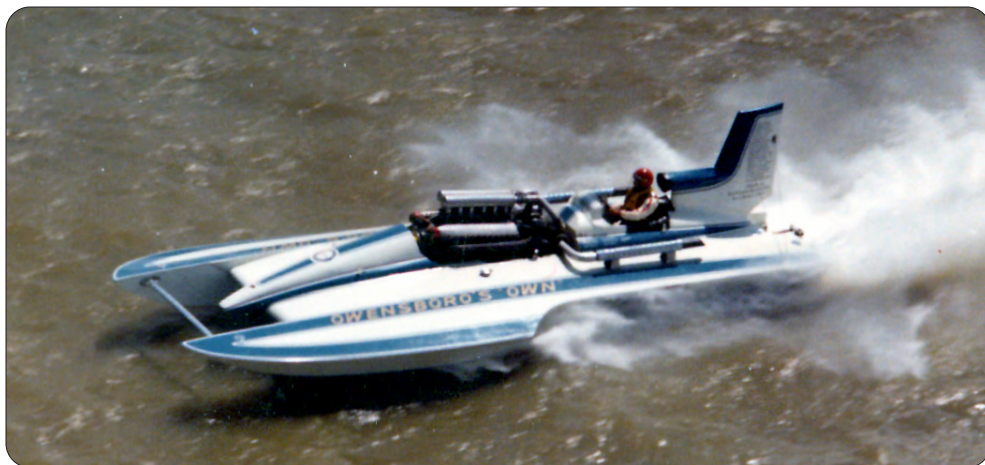
After the 1974 season, Walters was tasked with the job of converting the Red Man to a conventional set-up with the cockpit behind the engine. The hull is shown here in 1975 racing as Owensboro's Own .
