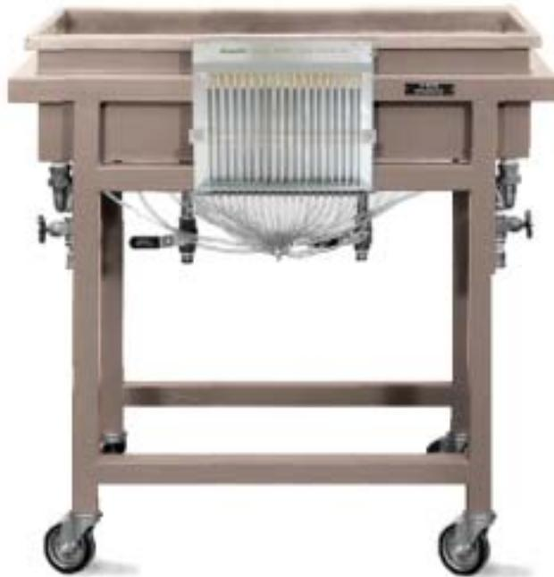
**MODEL H-6526** Ground Water Flow Tank
