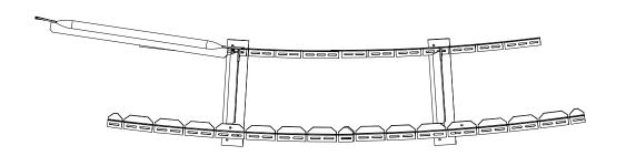
Sections of base and outer rings may be removed for clearance, – after the complete rings are finished
