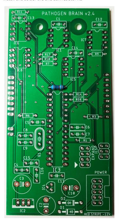
Install and solder the six 100K resistors R6, R7, R14, R16, R17 and R18
