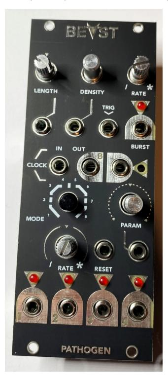
Install a few of the knurled nuts (I did 4) firmly and install washers and nuts onto the two round potentiometers – FINGER TIGHTEN only otherwise if you overtighten the potentiometers will lift off the PCBS and/or twist. This was enough tension to allow me to flip the board over to solder everything without it falling apart. Carefully test it out – you may need to install knurled nuts onto more jacks to get more tension.
