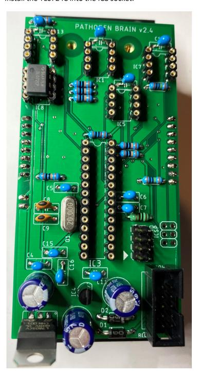
Install the four MCP602 IC's into their sockets (IC1, IC5, IC6 and IC7)
