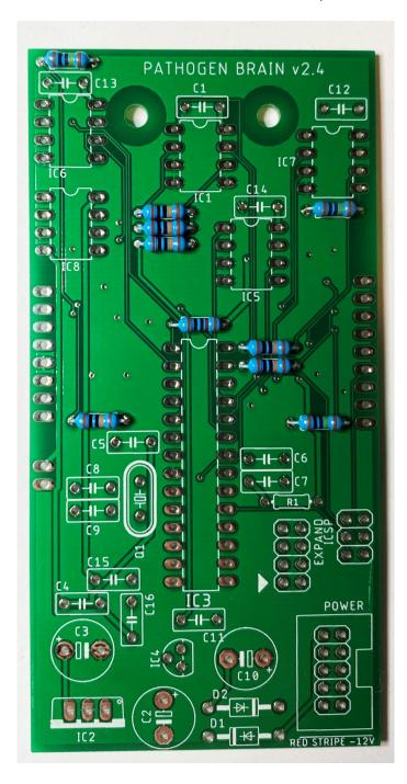
Install and solder the 100uh inductor into R1
