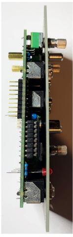
Install the remaining knurled jack nuts and potentiometer washer/nuts. Now that the potentiometers are soldered in tight, you can tighten the nuts but don't go overboard. Double check everything is seated correctly then flip over and solder the rest of the pins.
