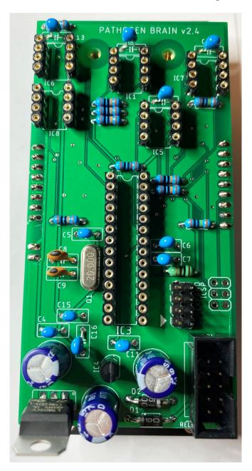
Install the TL072 IC into the IC8 socket.
