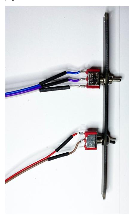
Slide the heat shrink tubing down over the lugs and use a cigarette lighter or heat gun to shrink the tubing into place.
