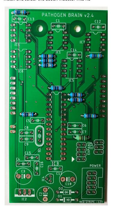
Install and solder the two 1N4004 power diodes into D1 and D2 paying attention to the polarity indicated on the silk screen.
