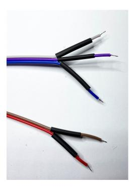
Solder the 3-wire piece onto the ON-OFF-ON switch. Solder the 2-wire piece onto the middle and top lugs of the ON-ON switch
