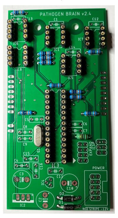
Install and solder the two 22pf capacitors into C8 and C9
