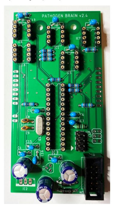
Install and solder the two voltage regulators IC2 and IC4, paying attention to the orientation marked on the silk screen.
