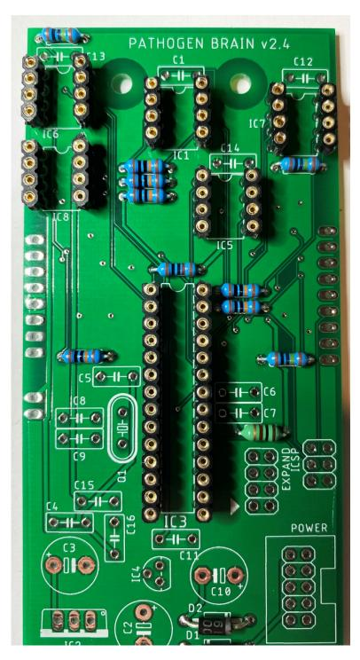
Install and solder the 20mhz crystal into Q1
