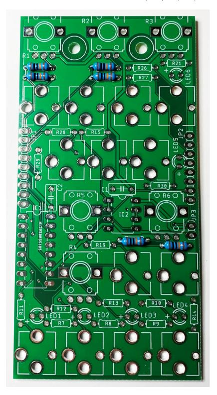
Install and solder the five 220R resistors R7, R8, R9, R10 and R21
