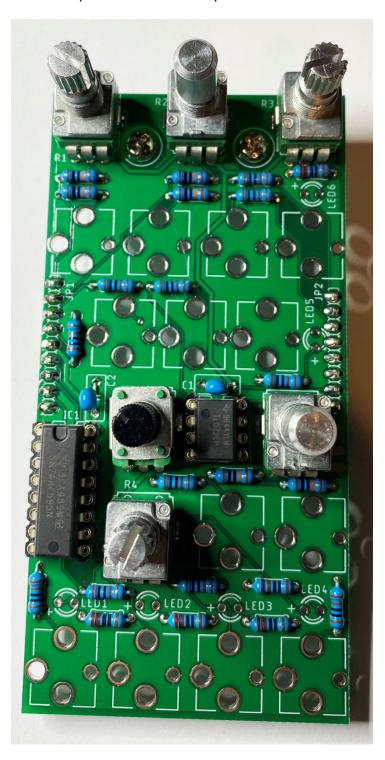
Seat the jacks (DO NOT SOLDER) and install the five red LEDs into LED1, LED2, LED3, LED4 and LED6 along with the bi-color LED into LED5. Again do not solder them yet. You may need to gently ben the pins on the LEDS to allow the board to rest on the desk unless you are using something to hold the PCB off the desk.
