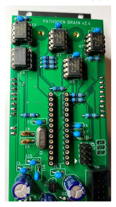
Install the Atmega CPU into IC3 and secure the boards together using the two remaining 6mm M3 screws.
