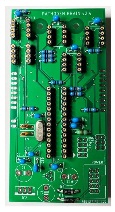
Cut two 4 pin pieces from the male pin header strip and install into the EXPAND header
