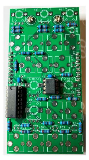
The trimmer pot needs its mounting supports trimmed in half so that they will fit into the PCB footprint. Use side cutters, go slow and be gentle.
