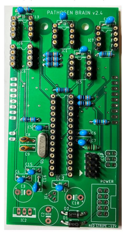
Install and solder the power header, paying attention to the cut out or "notch" indicated on the silk screen. Next install and solder the three 100uf electrolytic capacitors C2, C3 and C10 paying attention to the polarity. The longer pin is positive (anode) and the shorter pin marked with a strip is the negative (cathode)
