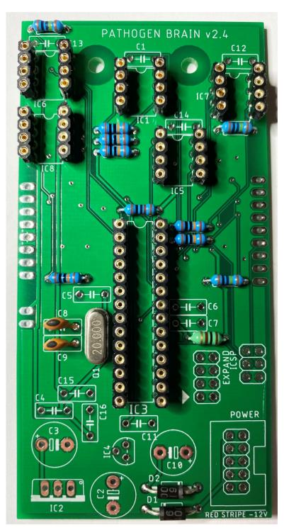
Install and solder the eleven 100nf capacitors into C1, C4, C5, C6, C7, C11, C12, C13, C14, C15 and C16
