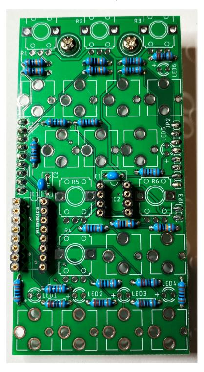
Install the 74HC595 IC into IC1 and the TL072 IC into IC2
