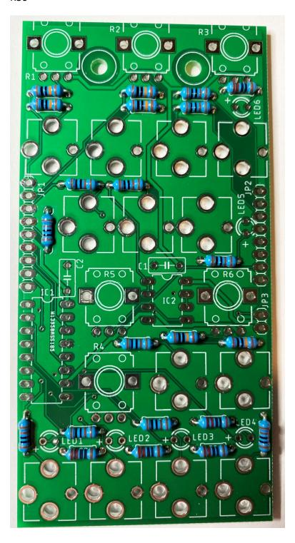
Cut IC sockets from the machine pin strips and install and solder them. Cut one 9 pin, one 8 pin and one 2 pin pieces from the male header pin strip and install and solder into JP1, JP2 and JP3
