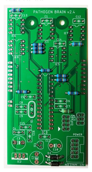
Cut the remaining IC sockets from the machine pin strips. Install and solder them into place.
