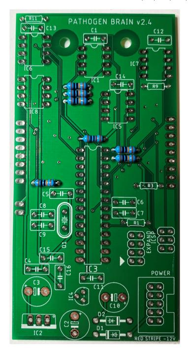
Install and solder the three 1M resistors R3, R9 and R11
