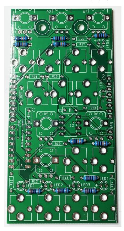
Install and solder the eleven 1K resistors R11, R12, R13, R14, R15, R19, R26, R27, R28, R29 and R30
