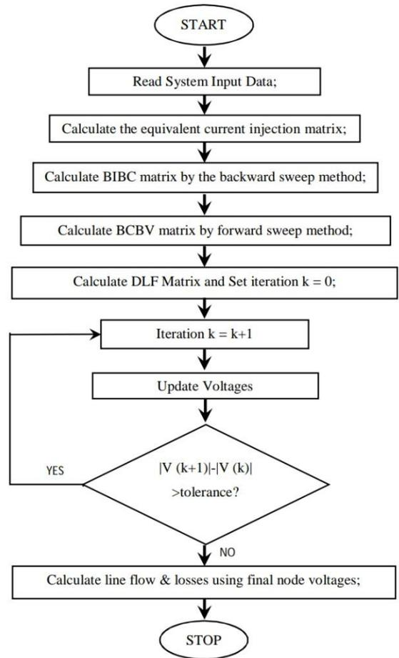
Figure 2: Flowchart for load flow solution for radial distribution networks.
