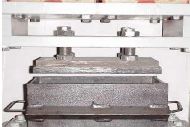
2. Place the white calibration block and two of the steel compaction plates into the steel mold.
