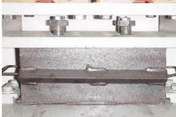
6. When the vibrating assembly base plate rests on the steel mold, tighten the four nuts on the top of the compaction head until they touch the compaction head.
