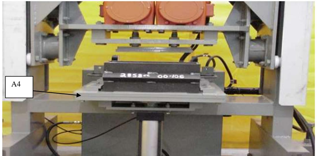
Figure 3. Beam Specimen Compaction Head
