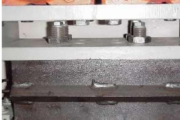
7. Raise the compactor and tighten the four remaining nuts under the compaction head.
