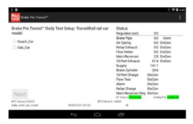
Once the car model has been selected, the program will guide the operator through setting up the device for the test, including making all hose connections.
