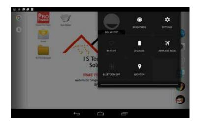
Once the Brake Pro Transit™ application has started and connected to the testing device, and an Operator ID has been entered, the Main Menu will appear. The Bluetooth Status in the lower right column will read Connected in green.
