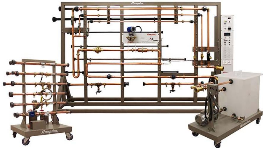
Shown **Model H-6920-CDL** with optional **H-6920-MR** Mobile Storage Cart (left) for storage of Sensing and Transmitting accessories. Also shown, optional **H-6920-22** Water Pump system (right).
