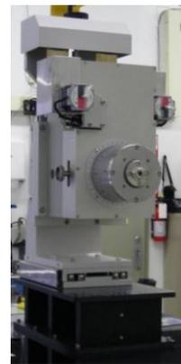
Figure 3: Dual-axis high precision goniometer
