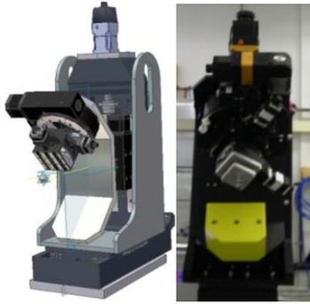
Figure 4: Single-axis inclined goniometer (CAD & photo)
