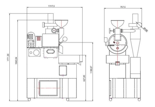
(These models have stands as seen in drawings below) Therefore you will need to adjust total length of exhaust pipe going out of building based on height of pipes of roaster.
