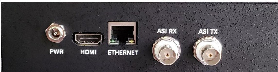
1. Power: Supplied by 5VDC 3.6 amp external power supply provided with unit. Redundant power supply optional.
