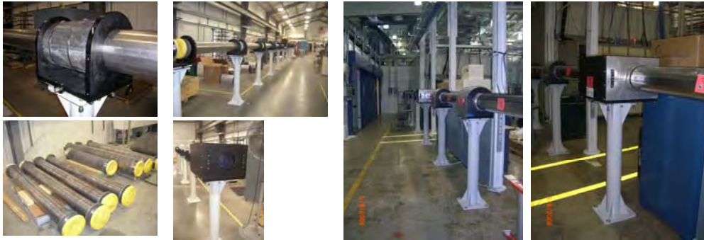
Shielded transport pipe with shielded stand assembly for Advanced Photon Source (APS)
