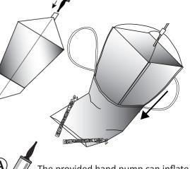
Inflate the Solar Balloon using a pump  $(\mathbf{A})$ , a large plastic bag  $(\mathbf{B})$ or, as a last option, by mouth. The corners of the Solar Balloon should remain soft. Remove the straw. **DO NOT over inflate!**
