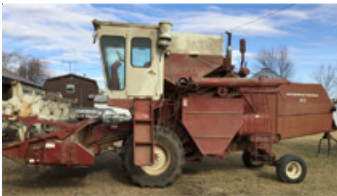
IH 615 Combine w/quick disconnect 13' grain head John Deere 343 Corn head 3 row-30"
