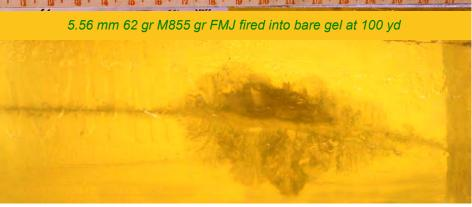
Two other yaw issues: Angle-of-Attack (AOA) at impact variations between different projectiles, even within the same lot of ammo, as well as AOA variations caused by differences rifles--referred to as Fleet Yaw, were elucidated by the U.S. Joint Service Wound Ballistic Integrated Product Team (JSWB-IPT) during their landmark studies from 2002-2006.
