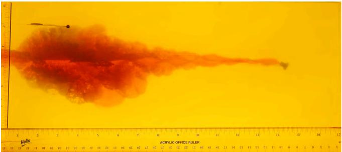
5.56 mm BH 50 gr TSX OTM fired into bare gel at 3 m from 10.5" barrel
