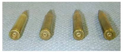
However, despite what appeared to be good primer strikes, two problems were discovered. First, when accurately measured, some of the primer strikes had insufficient firing pin indentations due to faulty weapons. The failed round from the potential OIS incident had a primer strike of only .013"—the minimum firing pin indent for ignition
