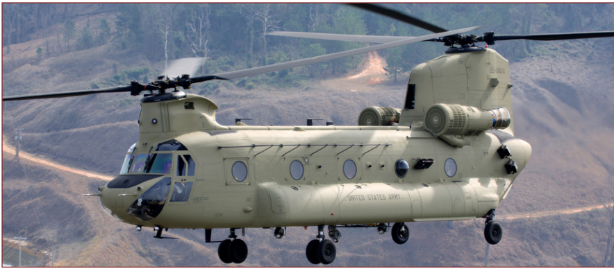
The Boeing Ch-47 Chinook helicopter was powered by the Lycoming T-55 turbine.
