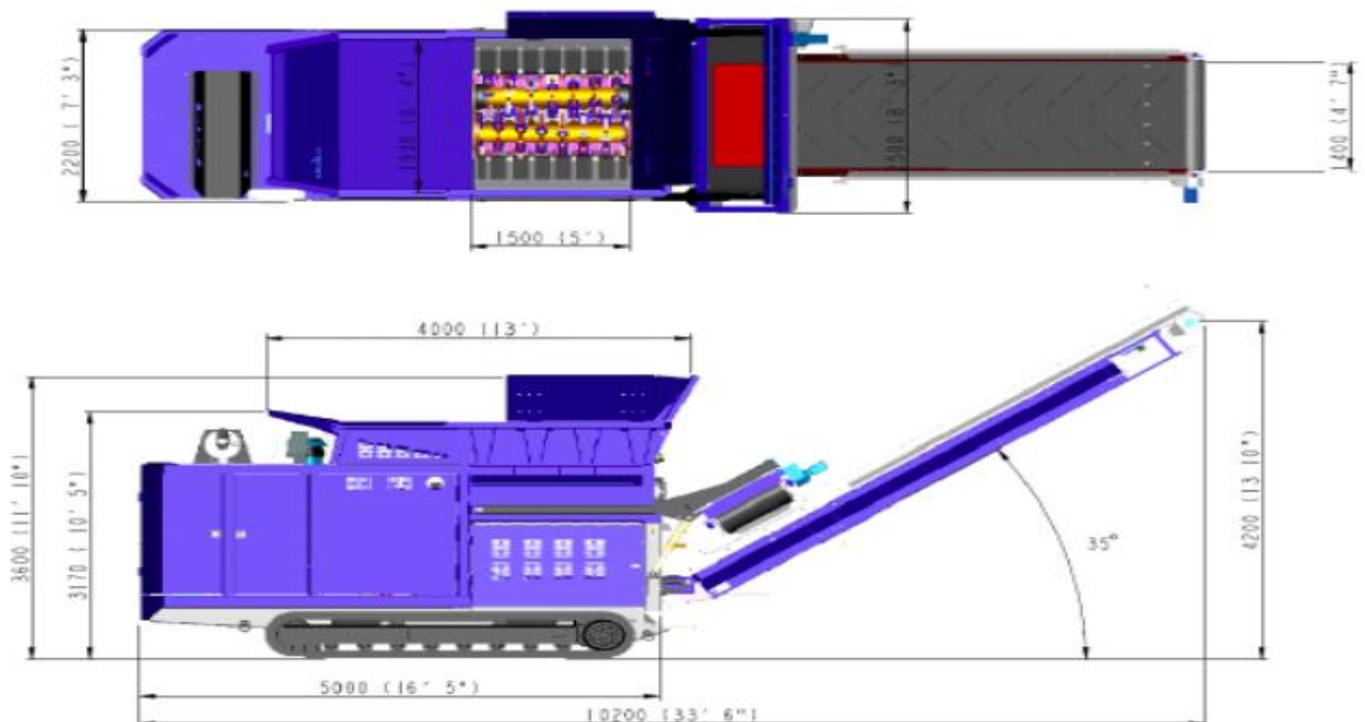
The shredded machinery conveyor feeds the shredded waste directly onto the trommel's in-feed system as part of the next treatment stage.
