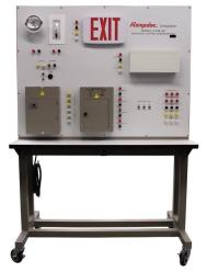
The **Model H-EM-2D** includes the following: Load Center, Control Console, Nickel-cadmium Battery, Battery Charger, Distribution Panel, Remote Control Alarm, Exit Sign Fixture, Flood Light and Wall Fixture.
