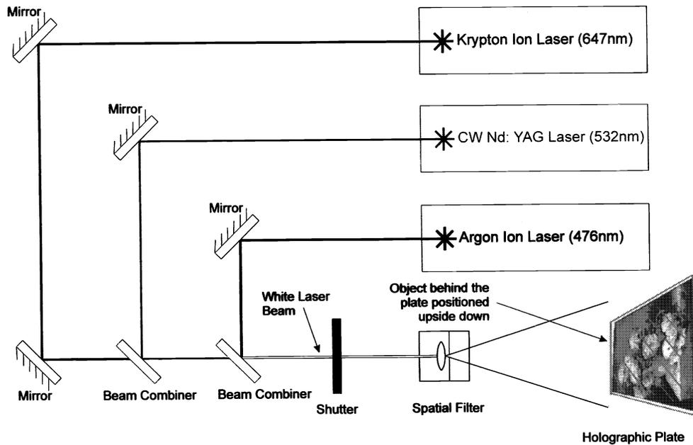
Fig. 1: Setup for recording a color hologram of a painting.
