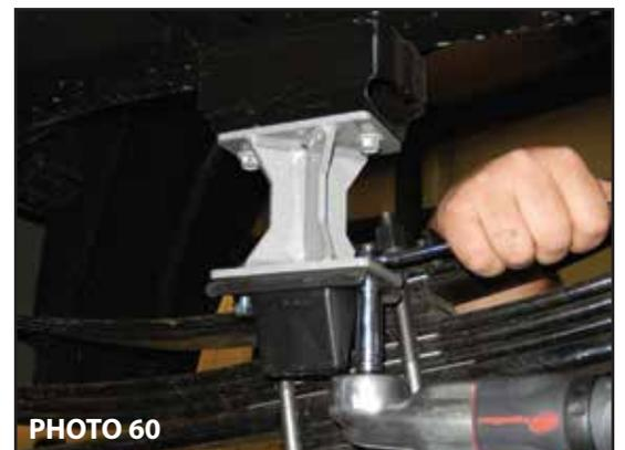
71. Install the McGaughy's brake line bracket with the stock stud and 9/16" nut. Position the bracket so the bend comes over the axle. (Photos 60 & 61)
