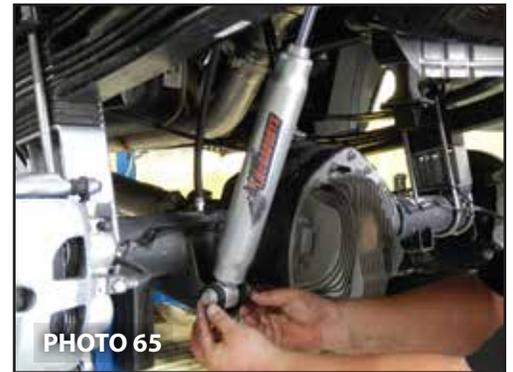
74. Install the new shock with body down. (Photo 64)
