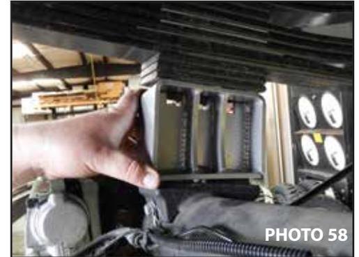
64. Insert the supplied 4 1/2" lift block with the tapered side facing forward. (Photo 58)
