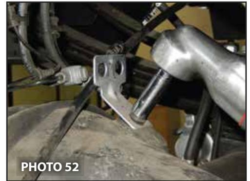
57. Remove the bracket to axle stud using a 9/16" socket. (Photo 52)
