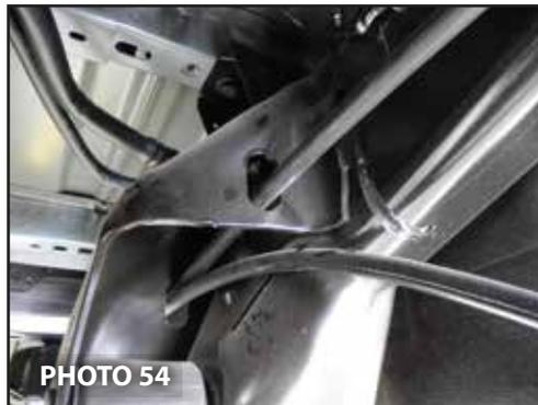
59. Pull the parking brake cable through both holes in the cab mount and front leafspring hanger. (Photo 54)
