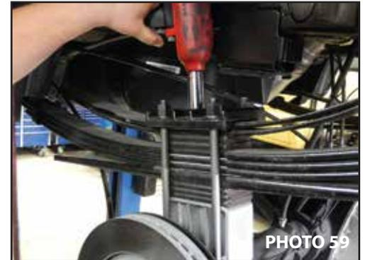
70. Install original bump stop onto new McGaughy's rear bump stop bracket using provided 3/8" hardware with lock nut and tighten down. Reinstall new mount back onto frame using original hardware as shown in Photo 59.
