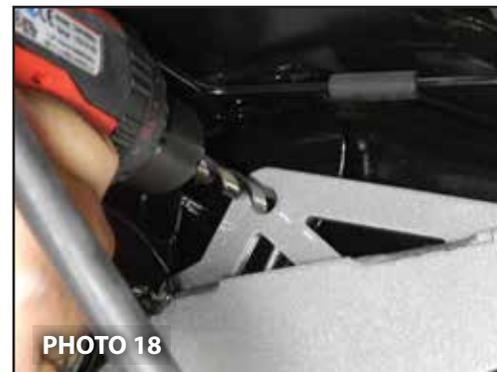
20. To mount the McGaughy's track bar relocation bracket, start by placing the factor bolt through the track bar bracket and drill the brace hole using a 7/16" drill bit. (Photo 17 Place something firm between the crossmember and oil pan to prevent damage. **NOTE: The top hole on the bracket may or may not require drilling with a 1/2" drill bit, due to the production variances on Ram frames.** (Photo 18)
