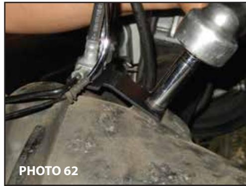
72. Mount the parking brake cable onto the stud using the factory hardware. (Photo 62)
