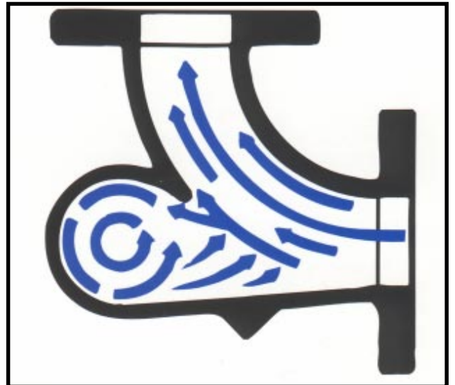
Flow characteristics of Smart Elbow™ prevent plugging.
