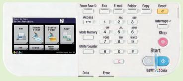
bizhub C35 is extremely simple to operate with an easy-to-see 32,000-colour high-resolution LCD display, easy-to-use large buttons, and icons that are recognisable at a glance.
