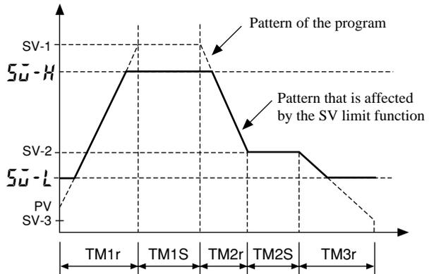
[Setting example] Setting the 1st target SV to 400°C
