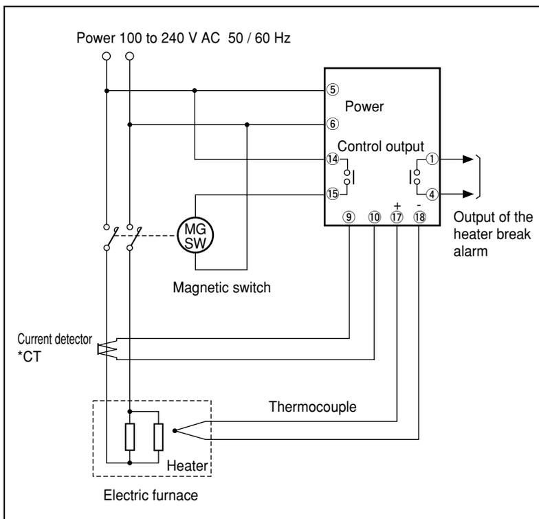
• How to connect the current transformer (CT) for heater break:
