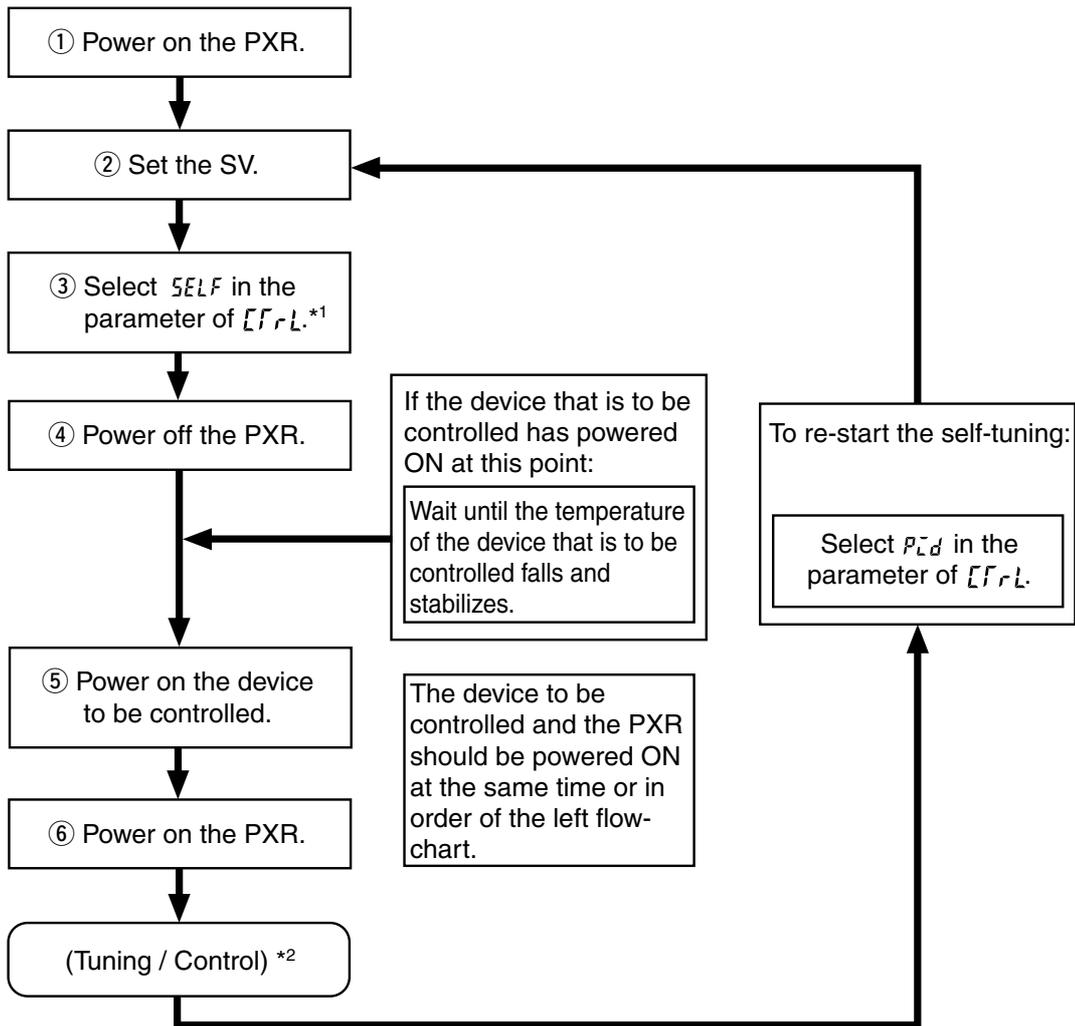
\*1: How to set the parameter of CFrL:
