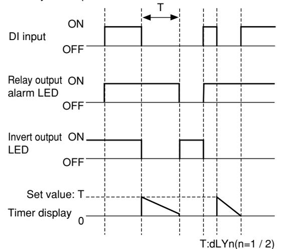
[Setting example] Setting the delay time for ON-delay alarm to 30 seconds
