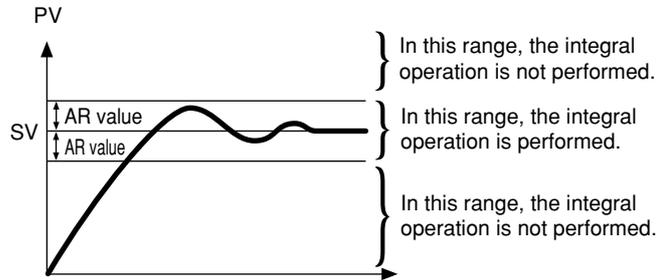
[Setting example] Changing the anti-reset windup from 60°C to 80°C.
