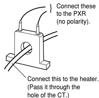
[Setting example] Changing the detecting current of heater break from 8.0 A to 9.0A
