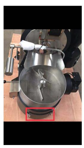
1. If you want to replace the mixing motor, first open the door under the cooling tray.
