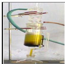
Fig 2: Soxhlet extraction
