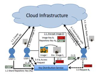
Fig. System Architecture
