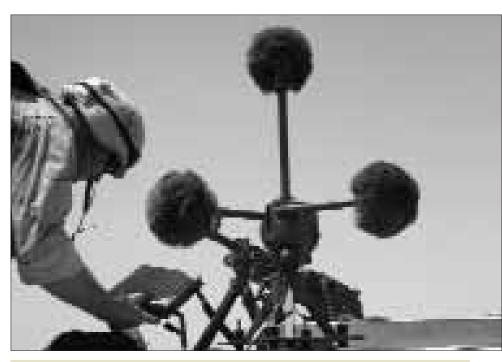
**Gunfire Detection System.** This device quickly detects and locates the origin of small arms fire, allowing troops to rapidly return fire and enhancing their survivability.
