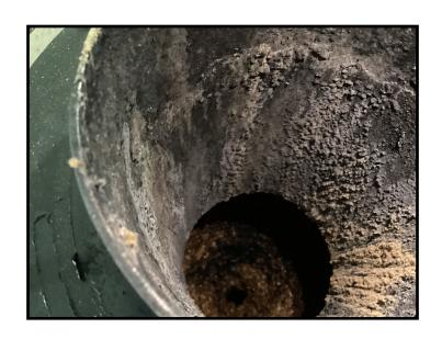
CHAFF FAN NOT CLEANED AND MAINTAINED: EXPECT TO REPLACE PARTS DUE TO FAILURE TO CLEAN
