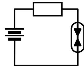
Circuit diagram for determining ignition curves
