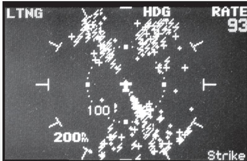
When cell mode is selected, a software algorithm kicks in that removes many of the strikes protruding out toward the aircraft in an attempt to eliminate the radial spread. This leaves the pilot with a much improved picture of where the actual cells are truly located.
