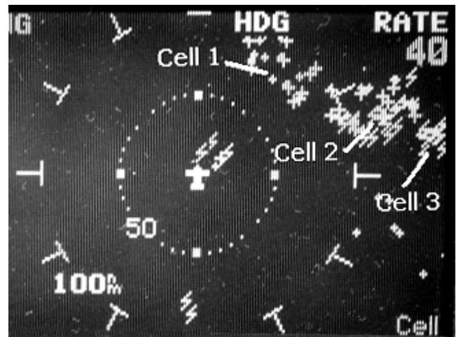
Radial spread is not necessarily always a bad thing. You can use it to your advantage to distinguish between false or clear air strikes and a real thunderstorm. Most of the strikes of a real storm will be of the average strike signature and be placed appropriately. As mentioned above, stronger-than-average strikes will be painted closer to the airplane.
