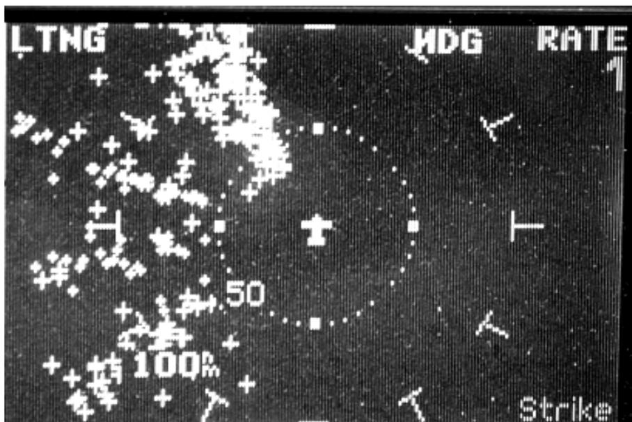
**Right:** Three cells are clearly visible in the air and on the Stormscope. Cell number three has almost all recent strikes, cell number two is a mixture of new and old strikes, and cell number one has mostly older strikes. This is a common pattern when cells form along a line of thunderstorms.
