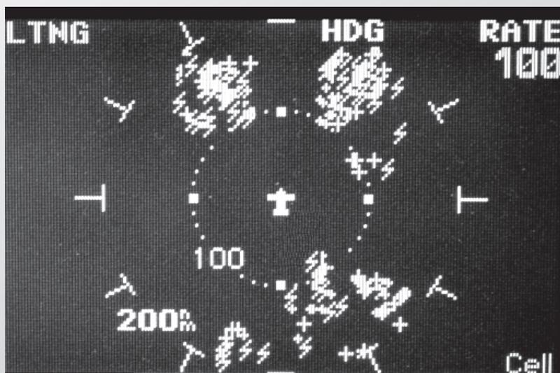
are displayed where the actual cell is located, but you may see dozens of strikes literally splattered all around the aircraft's location normally in the shape of a pie wedge.
