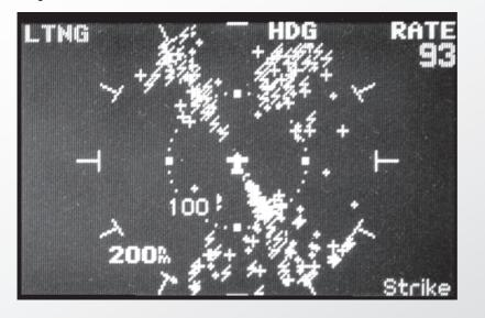
When cell mode is selected, a software algorithm kicks in that removes many of the strikes protruding out toward the aircraft in an attempt to eliminate the radial spread. This leaves the pilot with a much improved picture of where the actual cells are truly located.
