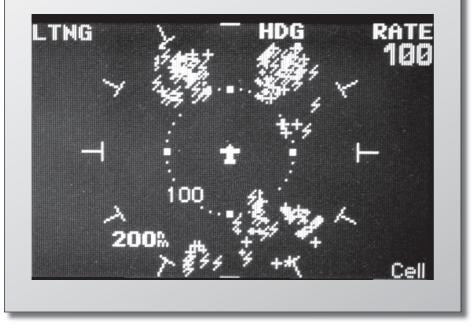
are displayed where the actual cell is located, but you may see dozens of strikes literally splattered all around the aircraft's location normally in the shape of a pie wedge.
