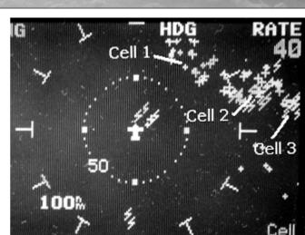
Radial spread is not necessarily always a bad thing. You can use it to your advantage to distinguish between false or clear air strikes and a real thunderstorm. Most of the strikes of a real storm will be of the average strike signature and be placed appropriately. As mentioned above, stronger-than-average strikes will be painted closer to the airplane.
