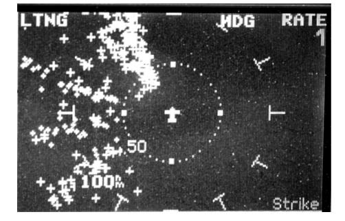
instantly detect the electromagnetic signals given off when lightning strikes the earth's surface. Cloud-tocloud and intra-cloud strikes are not detected.
