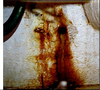
This is one of the telltales of crevice corrosion in through hull bolts. The fact that this is Taiwan stainless only makes the problem worse.
