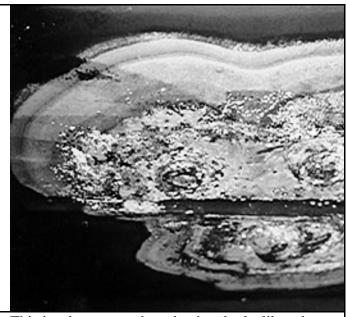
This is what copper-based paints looks like when stray current is involved with these through hull bolts. The copper-based paint has reacted. You can't get a better indicator of a problem than this.
